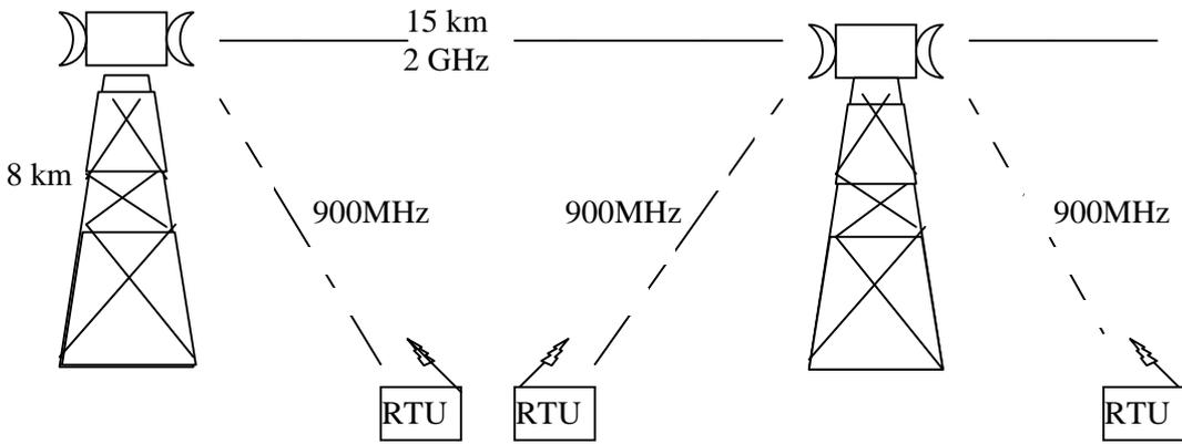
Figure 3: LAN Backbone system
