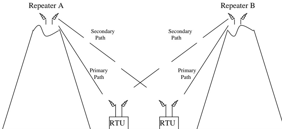
Figure 1: Repeater and comms path redundancy
