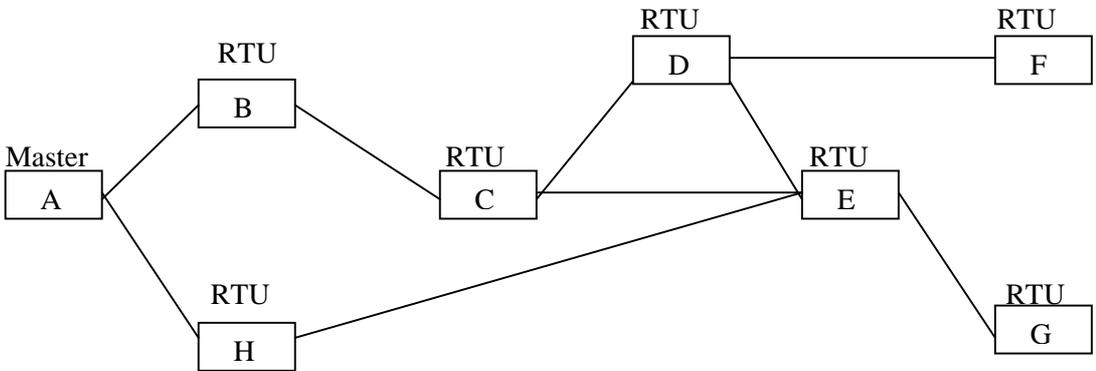
Figure 5: LAN telemetry system
